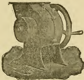
Machine for chopping ice used to pack about milk bottles.
